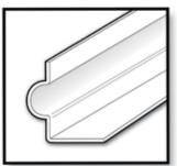
LocJoint is used where contraction joints are required in upper level lightweight concrete floors. This flexible lightweight PVC strip can be stapled to the wood substrate and will provide a weakened planed joint with a circular keyway that will interlock the division of the two slabs in unison.
